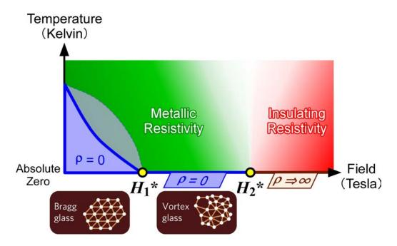
Research at Tokyo Institute of Technology and Florida State University has uncovered the whole picture of the *H-T* phase diagram and the complex interplay between vortex physics and quantum critical behaviour in lanthanum-strontium-copper-oxide high-temperature superconductors.
