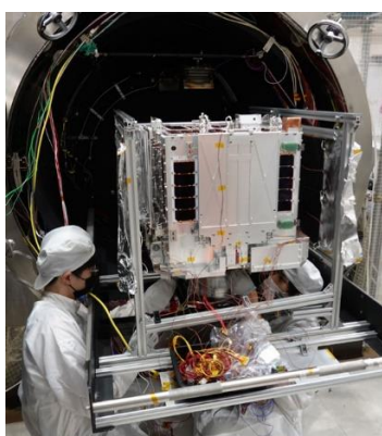
Figure 3. HIBARI satellite thermal vacuum test
