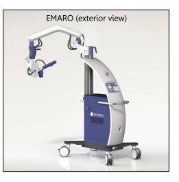
Until now, pneumatic manipulation technologies have not been able to provide the smooth and continuous movement needed for highly precise control of surgical devices. Professors Tadano and Kawashima overcame this hurdle by creating an advanced model with continuous air pressure control and an original manipulation technique. Their success owes much to Tokyo Tech Professor Toshiharu Kagawa, who had scored impressive results over decades of research in the field of fluid measurement and control.
