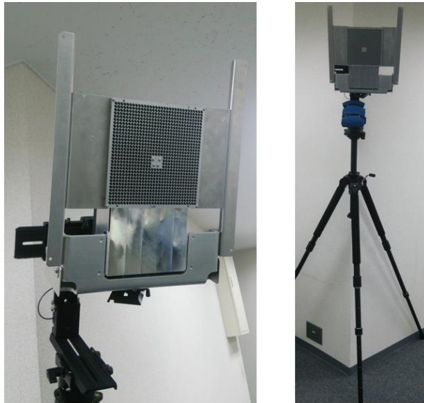
Fig. 3. Photographs of the 60 GHz GATE wireless system
