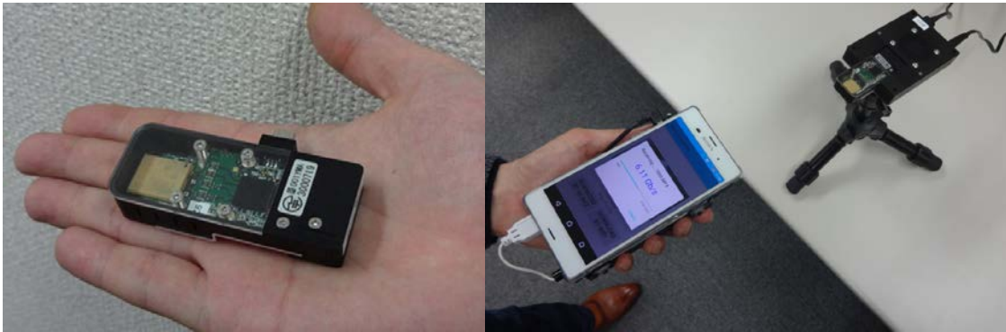
Fig. 2. Photographs of a 60 GHz 6.1 Gbps wireless module (left) and of experimental setup for wireless transfer of files to a smartphone (right)
