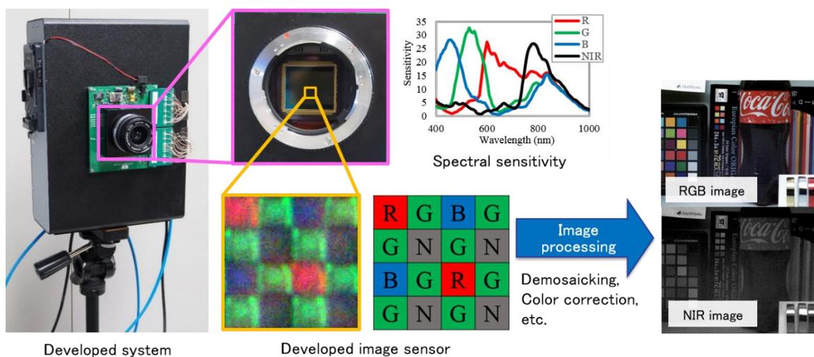
Figure 2 Overview of the developed prototype system.
