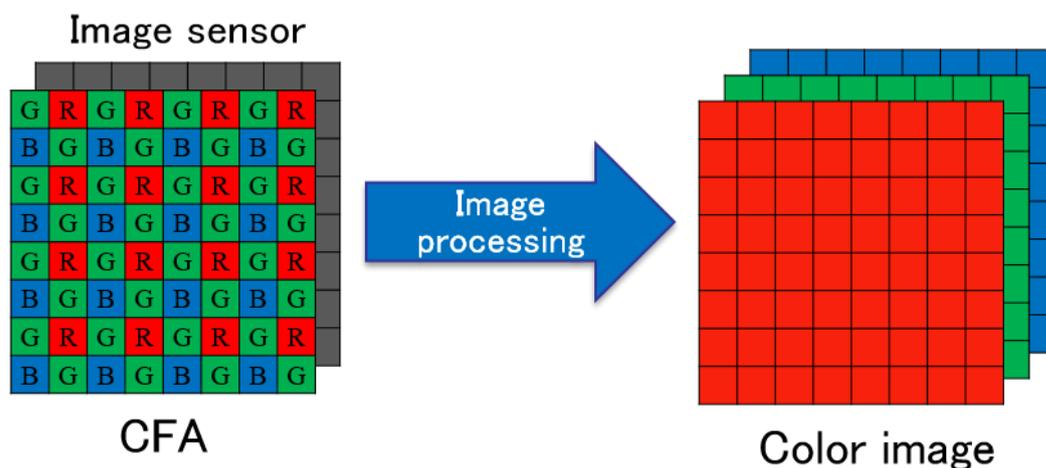
Figure 1 Color image acquisition using a single image sensor with a CFA.
