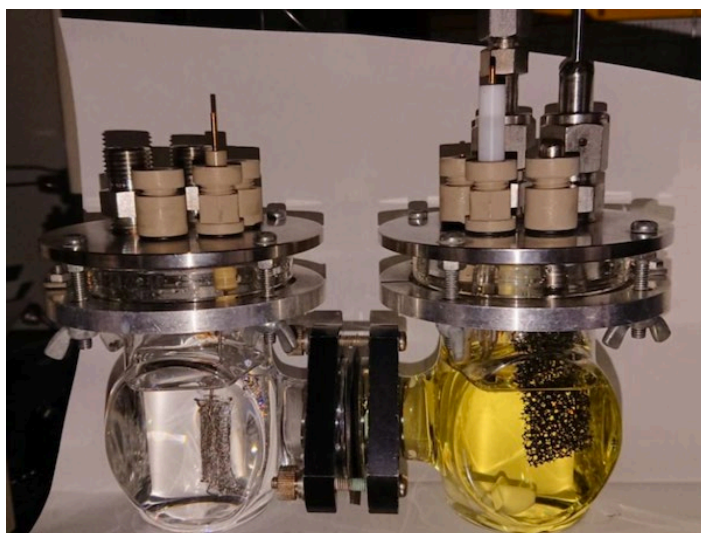
Figure 1. Photograph of the experimental setup for bulk electrolysis The CO 2 reduction reaction takes place in the cathodic chamber shown on the right.
