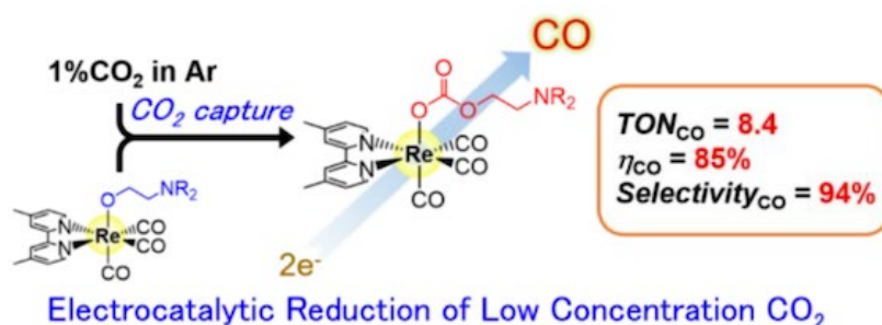
Figure 2. Representation of the electrocatalytic reduction system Electrocatalytic reduction of low-concentration CO 2 was achieved using a rhenium-based complex with high CO 2 -capturing ability.
