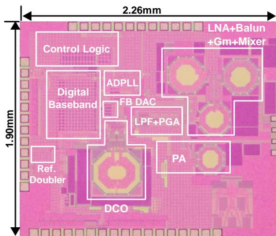
**Caption:** The chip was designed using standard 65-nanometer CMOS technology.
