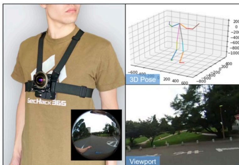
Figure 1. MonoEye captures 3D body pose as well as the user's perspective MonoEye is based on a single ultra-wide fisheye camera worn on the user's chest, enabling activity capture in everyday life.
