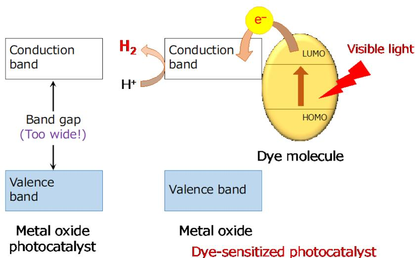
Figure 1. Dye-sensitized  $\text{H}_2$  evolution using a wide-gap metal oxide.
