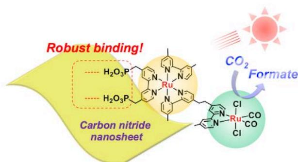
**Figure.** Schematic of solar fuel production by semiconductor photocatalyst. Researchers observed robust binding between the ruthenium metal complex and carbon nitride nanosheets under visible light in aqueous solution
