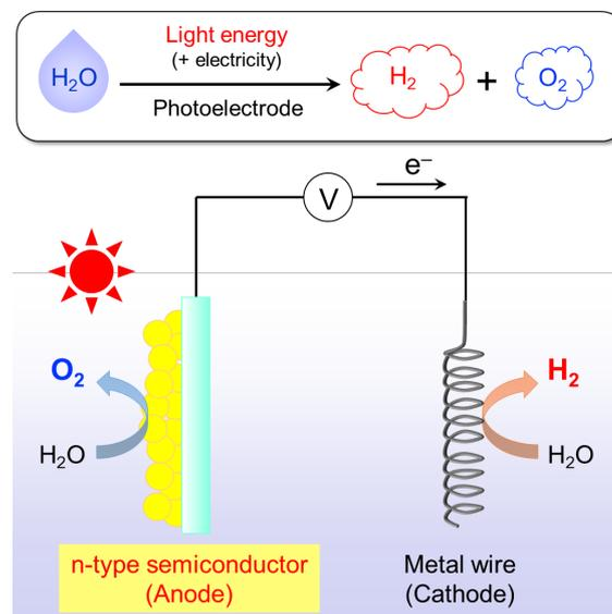
**Figure 1. Photoelectrochemical water splitting**
