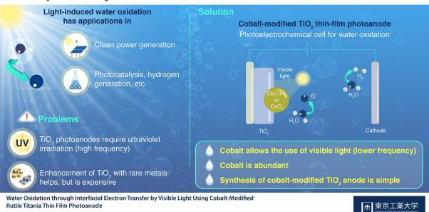
Photoelectrochemical water splitting, the process by which light energy is used to split water molecules into hydrogen  $(H_2)$  and oxygen  $(O_2)$ , is a promising approach to obtain pure hydrogen for use as an alternative clean fuel. This process is carried out in electrochemical cells that contain an anode and a cathode submerged in water, which are connected through an external circuit.
