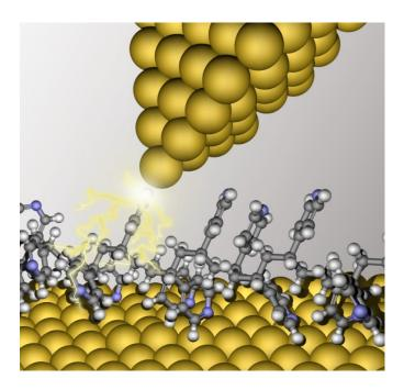
Figure 1. Single-molecule junctions composed of the STM tip and a polymer
