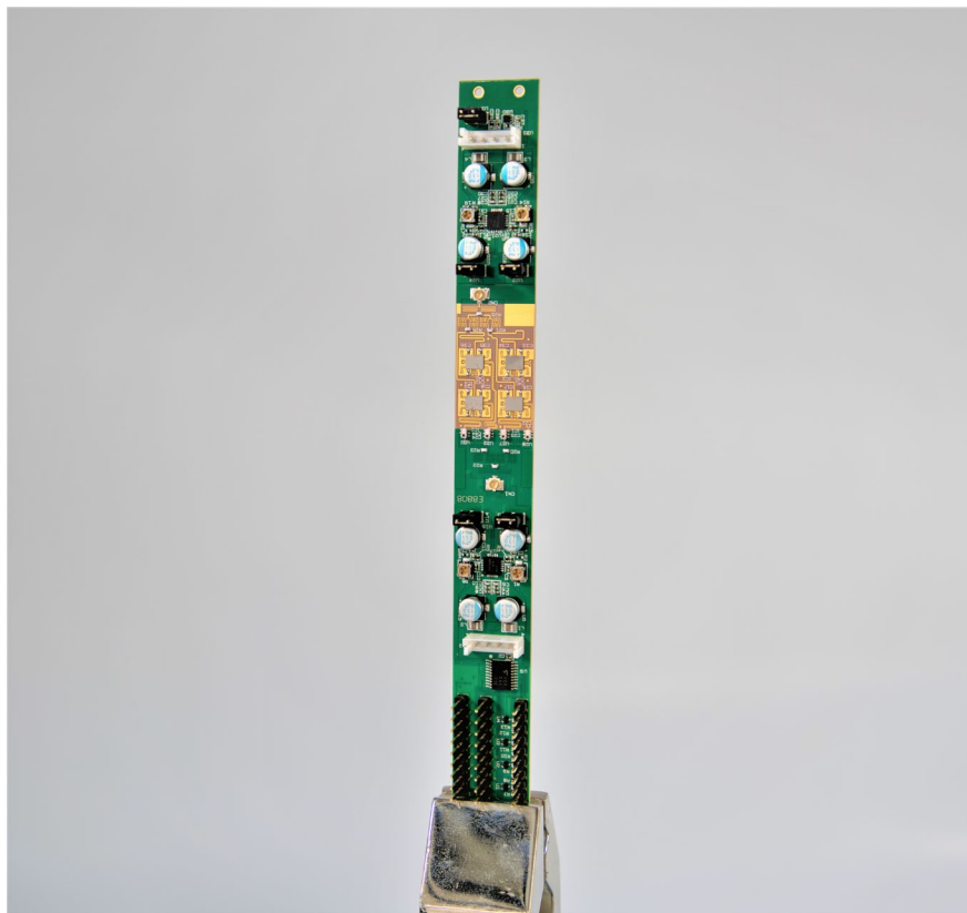
CMOS chips on an 18 mm x 163.5 mm evaluation-board
