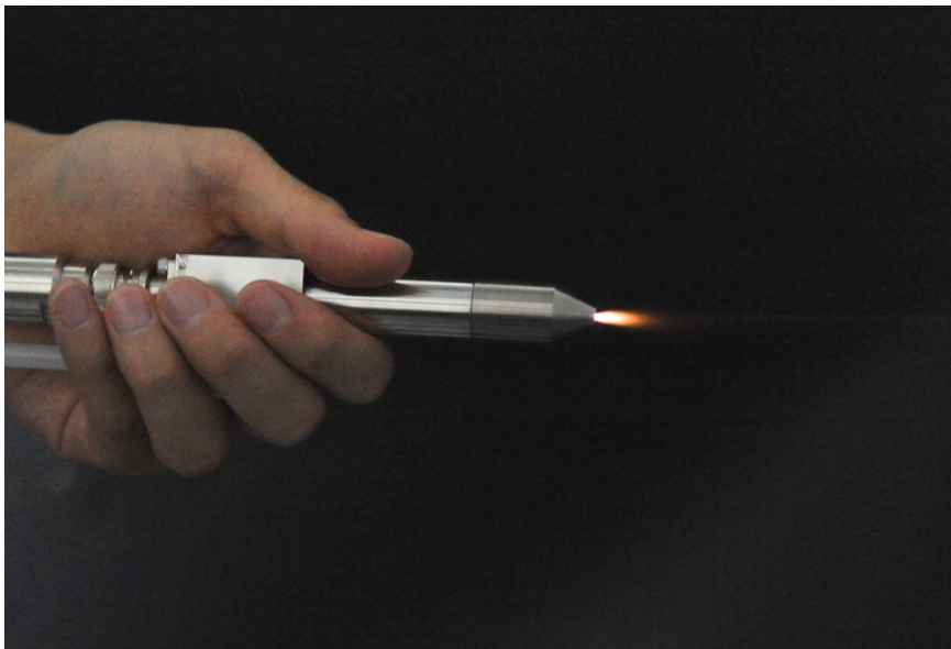
Figure2. Atmospheric low-temperature multi-gas plasma jet
