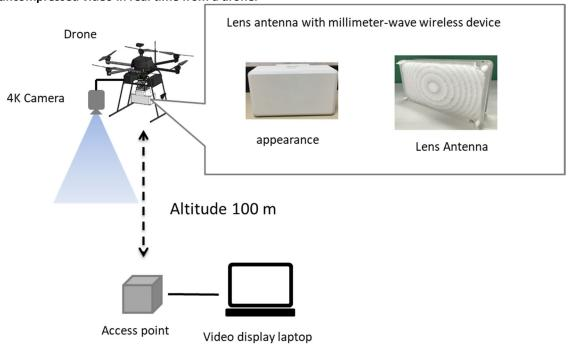
SECOM is focusing on services for securing wide area facilities by using wireless communication technology for drones. Wide area surveillance with drone requires real time transmission of high definition video such as uncompressed 4K videos providing the professional resolution, for rapid and accurate analyses.
