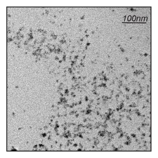
Title: Transmission Emission Microscope image of ZnS/hyperbranched polymer particles. Caption: The micrograph shows uniform nanoparticles under 10nm in diameter.
