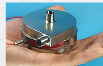
Implantable artificial heart using magnetic levitation
